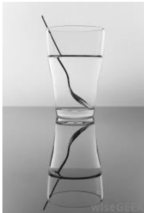
Figure 5. The effect of the speed of light. Because light travels slower in water than it does in air, rays of light bend (change direction) when they pass from air into water, or from water into air. In this case, light reflected from the spoon travels at a different angle through water than it does through air, making the spoon appear to be “broken” at the point where the water meets the air. (Image from WiseGeek: http://www.wisegeek.org/what-is-refraction.htm )
